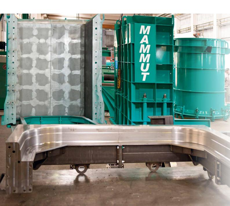
Mould cores, jackets, base pallets, spigot end shapers — all these elements belonging to the modular system reduce investment costs and increase production flexibility. MAMMUT moulds can be equipped with:
