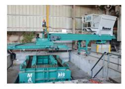
The hopper of the concrete feeder is filled via conveyor belt or travelling bucket.
