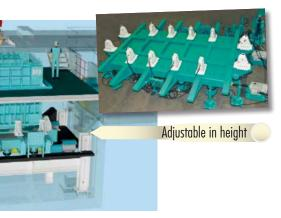
...the quick locking allows them to be moved freely over the table, enabling the production of different product sizes and types. The MAMMUT vibrating table is very stable and rigid, and is characterized by very smooth and powerful vibration, unfolding over the entire table surface. Here, the pneumatic controlled leveling system is used. As a result, the vibrating table's enormous power reserves can even cope with the biggest products.
