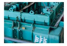
Customised designs are available for the spigot end. The spigot end is shaped under vibration, by eight hydraulic clamping cylinders integrated in the core. This production step is also completely automated. All parameters can be selected via the integrated touch screen.
