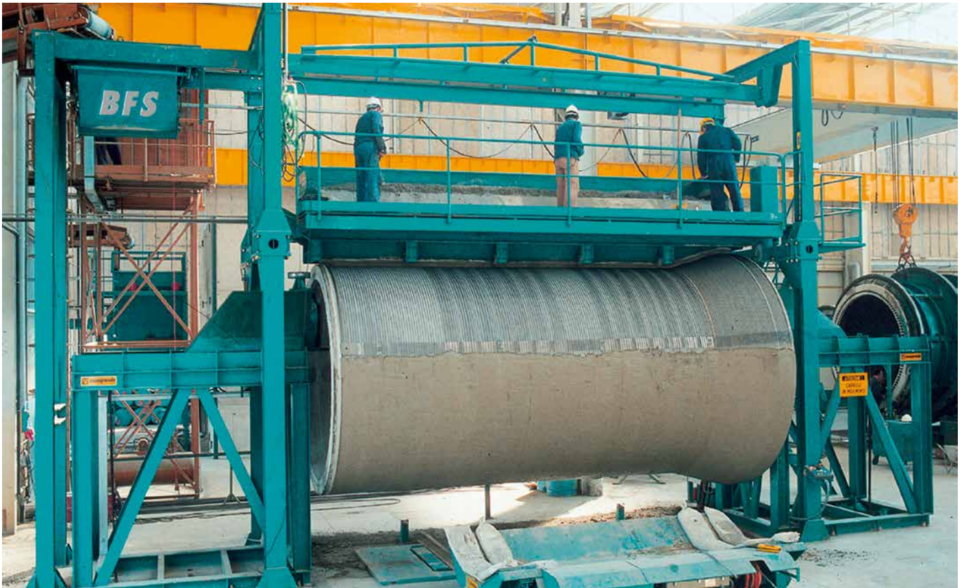
Mortar Coating Machine; in order to protect the steel wires against corrosion
