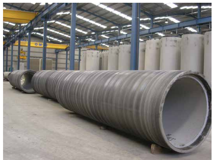
Radial Pre-stressed Concrete Cylinder Pipe
