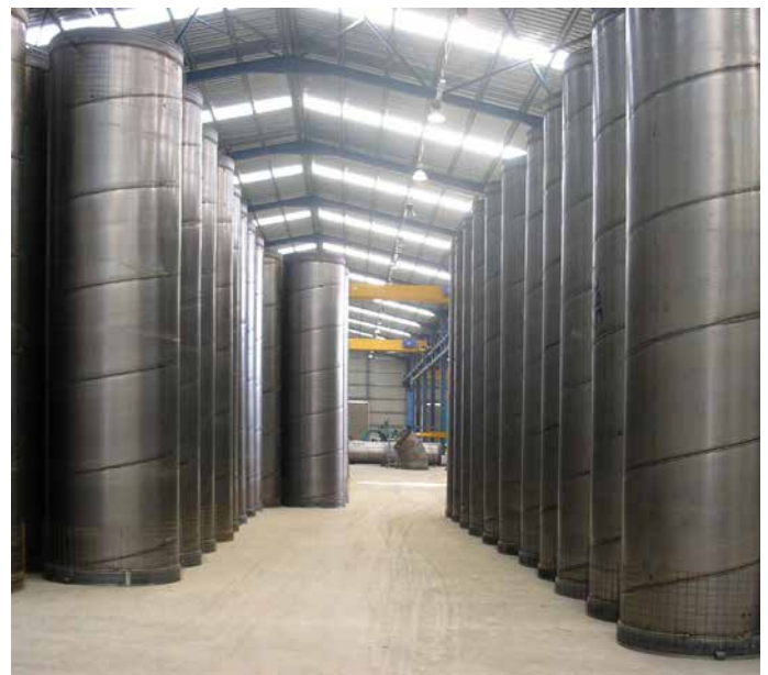
Steel Cylinders already tested against leakage and ready to be used
