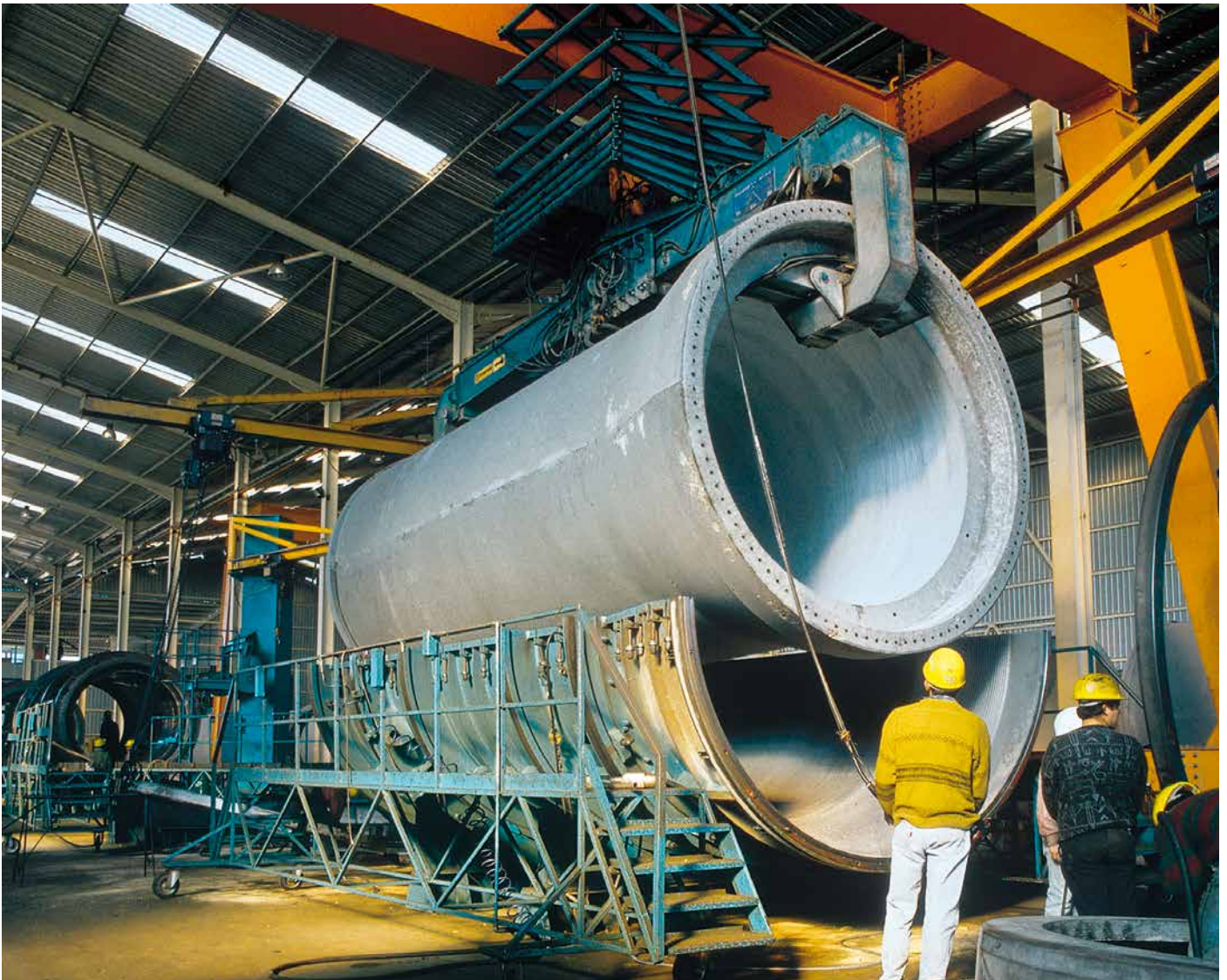
Demolding Process of a cured Pre-stressed Concrete Spun Pipe
