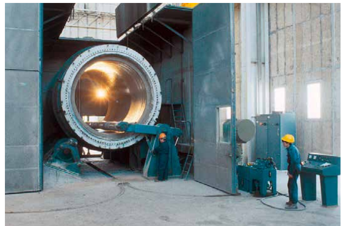
Concrete Pipe Spinning Machine
