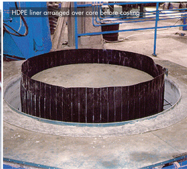
Hard liner in finished concrete pipes
